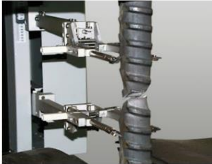
Figure (5): Tensile Test to Measure the Strength of Iron.
