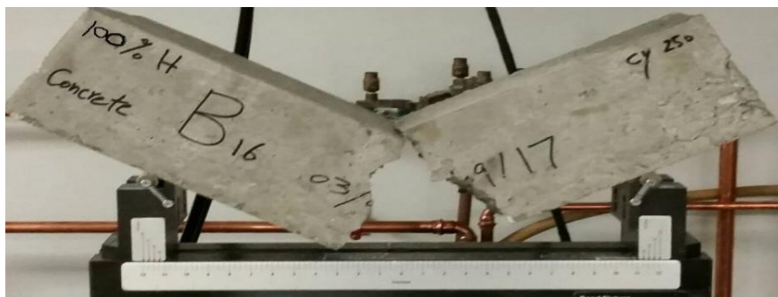
Figure (9): Flexural Failure of Concrete Beam-100% Relative Humidity.
