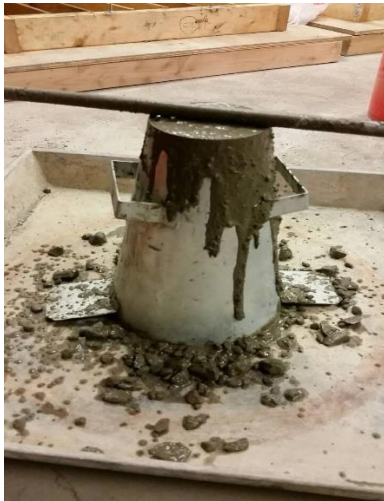
Figure (2a): Slump Test Cone Filled out by Concrete. Figure (2b): Measure the Slump Value.
