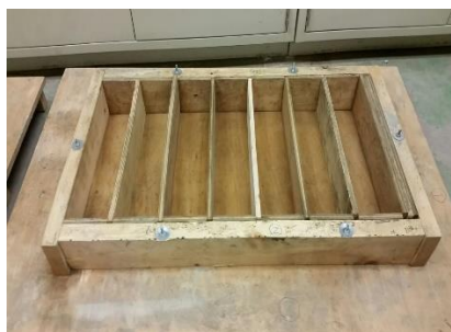
Figure (3): Rectangular Beam Moulds.
