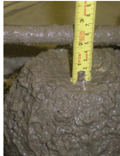
Figure (2a): Slump Test Cone Filled out by Concrete. Figure (2b): Measure the Slump Value.
