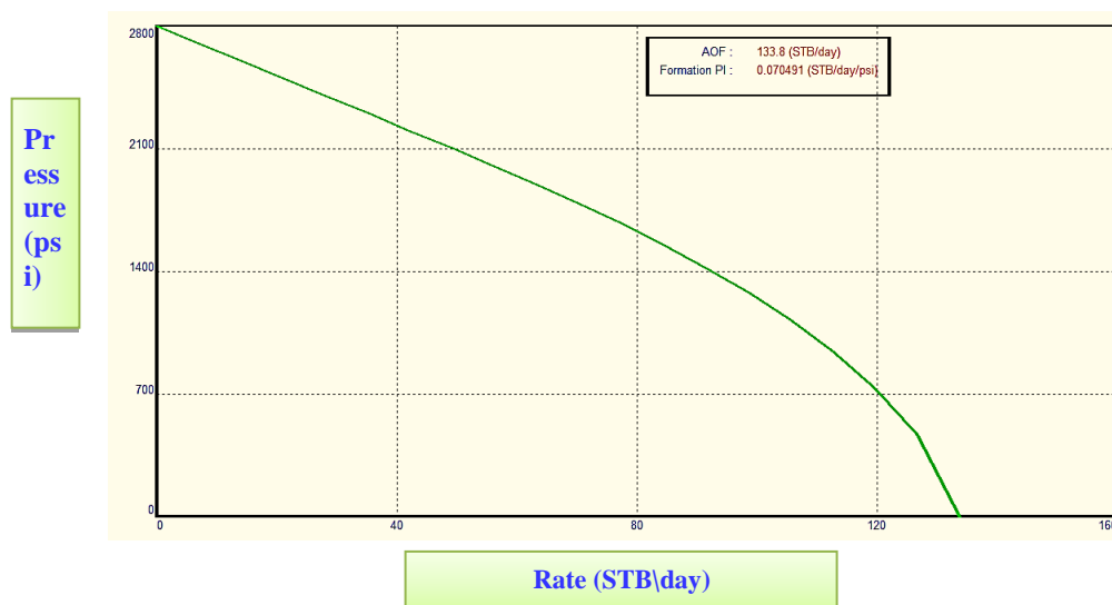
Figure (2): IPR Plot before Scale Removal for Well (B-96).
