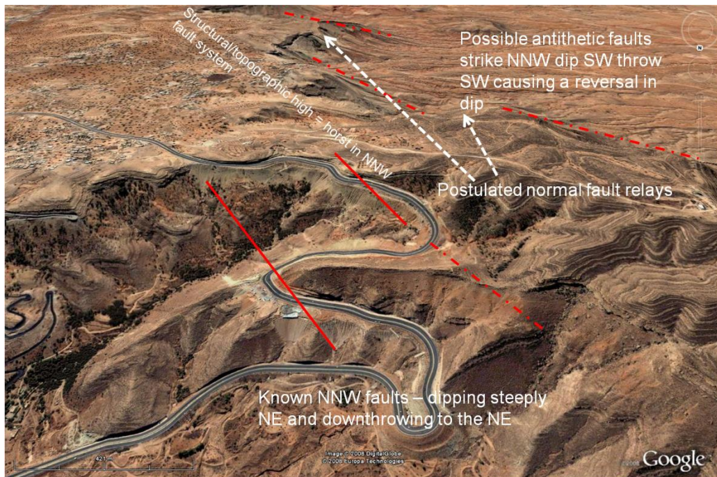
Figure (3): Front View of The Google Earth Satellite Image of The Landslide and Displacement in the Kiklah Formation Due to an NNW Fault Parallel to the Image.
